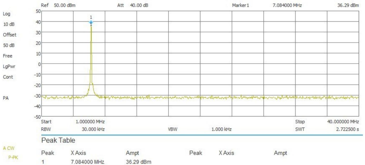
Figure 4 – Harmonics 40m at 5W of the IC-705
