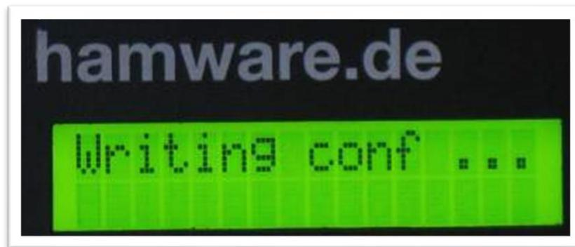
You can enforce the writing to the EEPROM using the button **Erase Memory bandwise** on the back-side of the AT-502:
