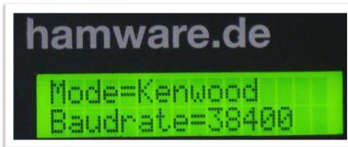
Use the rotary switch **L** for selecting the **Baudrate** of the transceiver serial interface.
