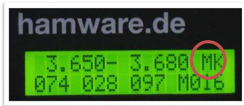
In this mode, only the right-most rotary **Manual** is active. It can be used to select the desired memory channel.
